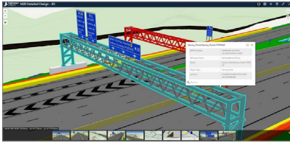
A view from the app showing the detailed design information and the ability to query it for BIM information.
