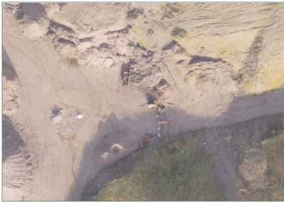
An orthomosaic model made from 700 images using Esri's Drone2Map
