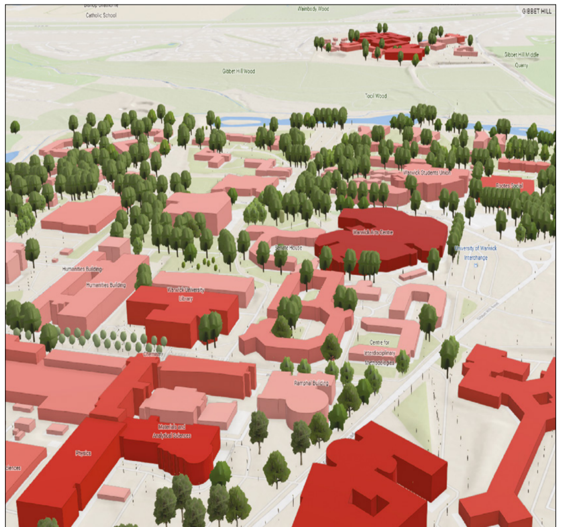
Buildings are colour coded according to energy consumption in the University of Warwick's 3D Digital Campus.
