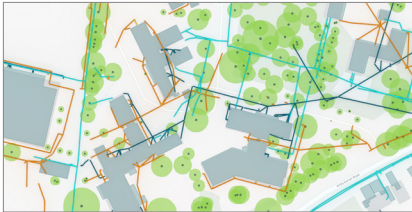
ArcGIS clearly shows the relationship between tree roots and underground services
